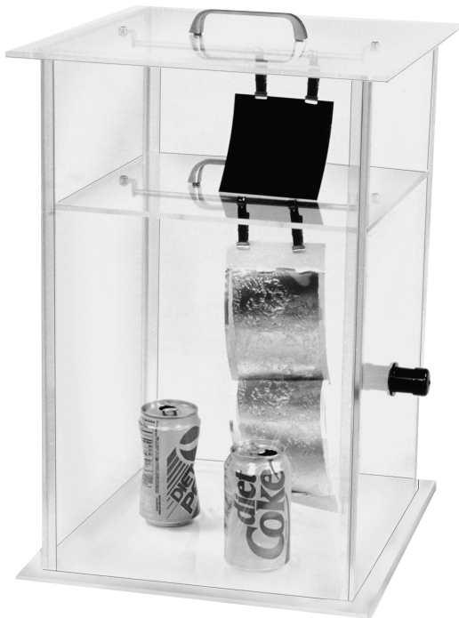
Figure 6–11 Superglue fuming in airtight box (also shown disassembled)..
