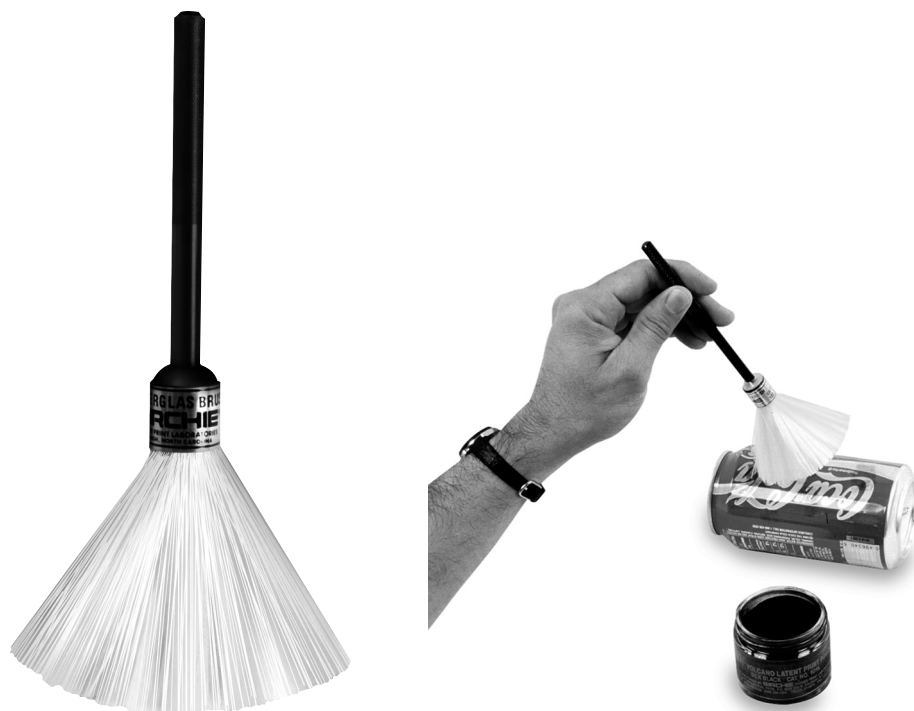
Figure 6-7 Fingerprint brush and use of brush to develop the print and remove excess fingerprint powder.
