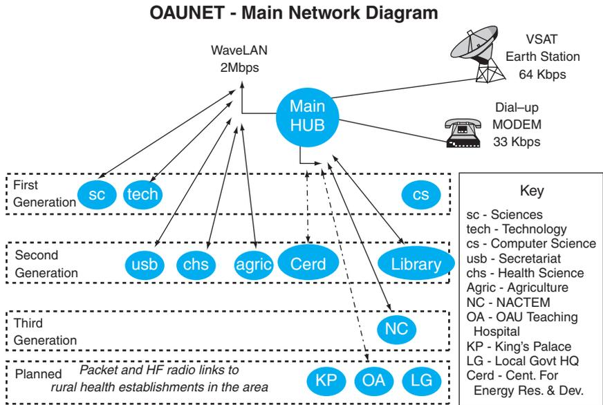
FIGURE 9-11 OAUNET in Nigeria: Main Network Diagram
