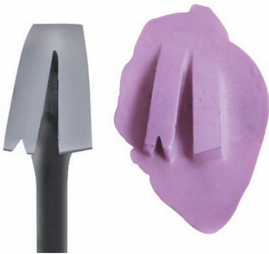
FIGURE 2-3 A cast of a hammer claw.
