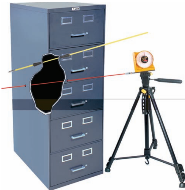
FIGURE 2-8 A laser trajectory finder is used to determine the path of a bullet.
