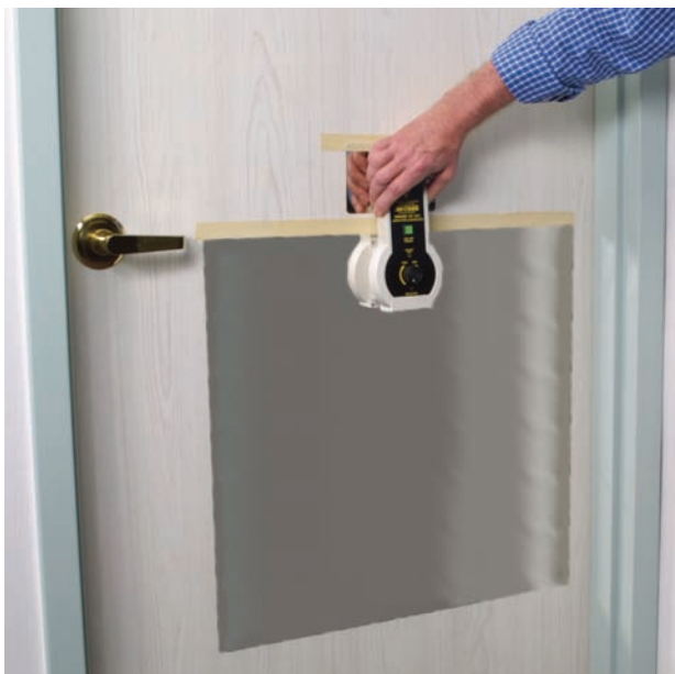
FIGURE 2-6 The electrostatic plate will lift dust from horizontal and vertical surfaces, thereby recording the impression.
