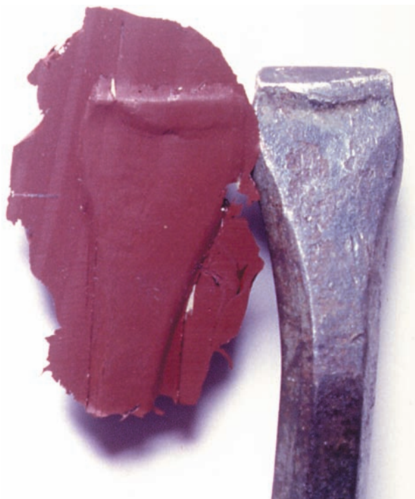
FIGURE 2-2 A cast of a tool mark.
