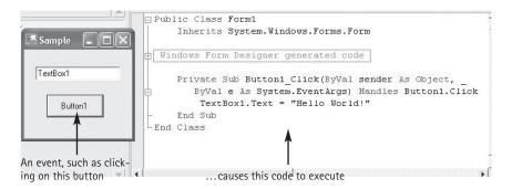
Figure 2-4 An Event "Triggers" the Initiation of a Procedure
