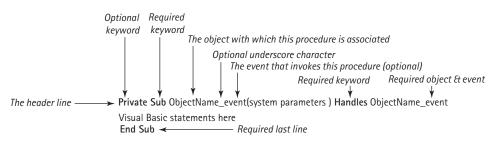
**Figure 2–19** *The Structure of an Event Procedure*
